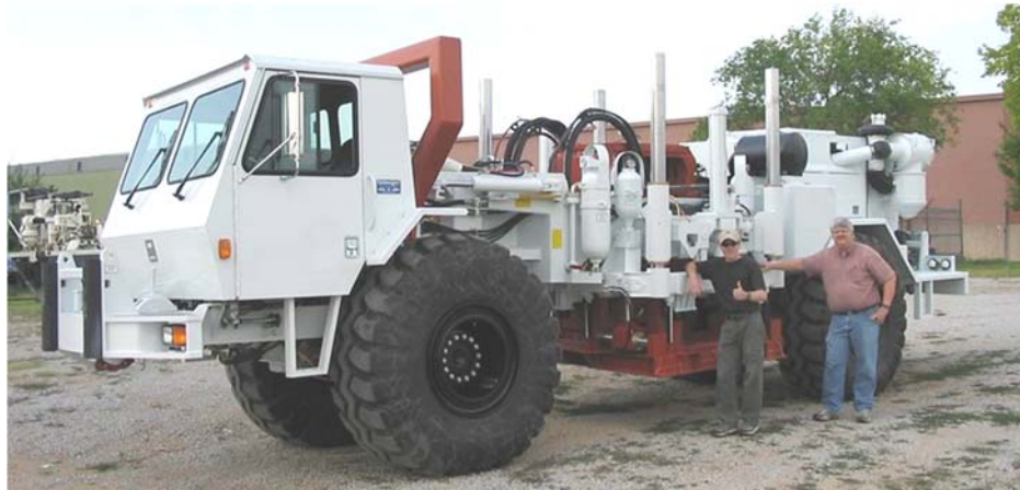
Low-frequency vibroseis, 64,000 lb-heavy Liquidator
